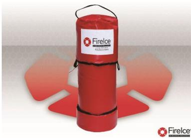
The Firelce Fire Extinguisher Heater Bag is designed to prevent the Firelce® inside the extinguisher from freezing during cold conditions. It automatically activates at 35 F and deactivates at 45 F. The heating element operates at 12 V DC-12 W-1 Amp.
