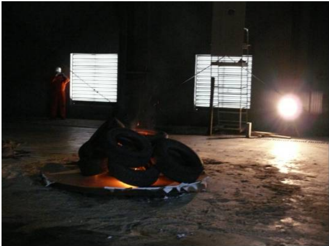
Figure A-8. Ten-Tire Fire at Initiation.
