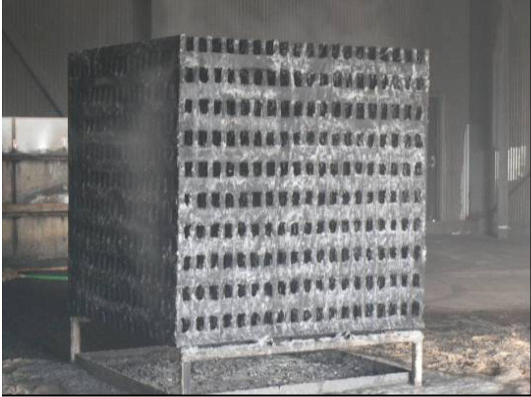
Figure A-7. Class 40-A Crib following Extinguishment.
